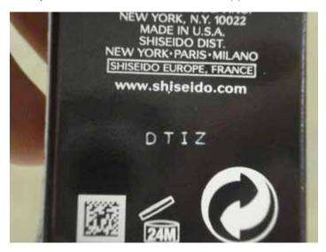
The small character continuous ink jet printers offer flexibility by being able to print both black and yellow inks, based on the color of the substrate. Mechanics handle the routine printhead cleaning on the continuous ink jet printers and related issues, like printer orientation and adjustments. The mechanics or line operators handle code generation, which is facilitated by a simple user interface.
